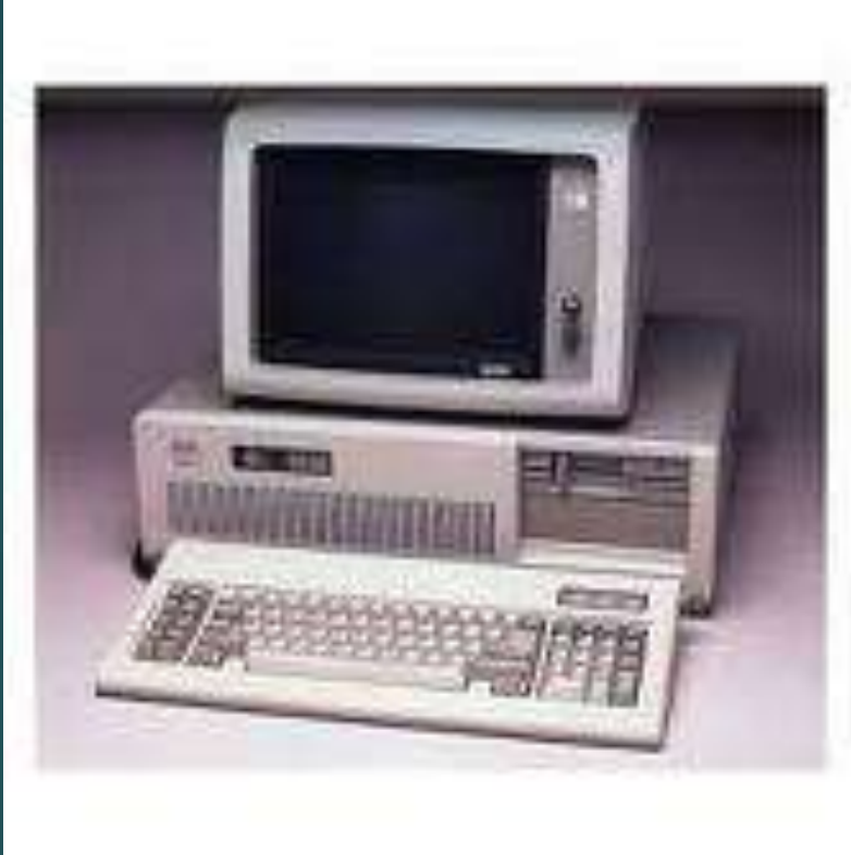
1982 IBM Computer Intel 8088 chip @ 4.77 MHz
